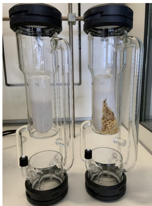
Figure 5. Cellulose cartridges initially filled with the same quantity of soybean seeds after a 2-h Soxhlet extraction with 2-MeOx (left) and 2-MeOx 95.5% (right).
